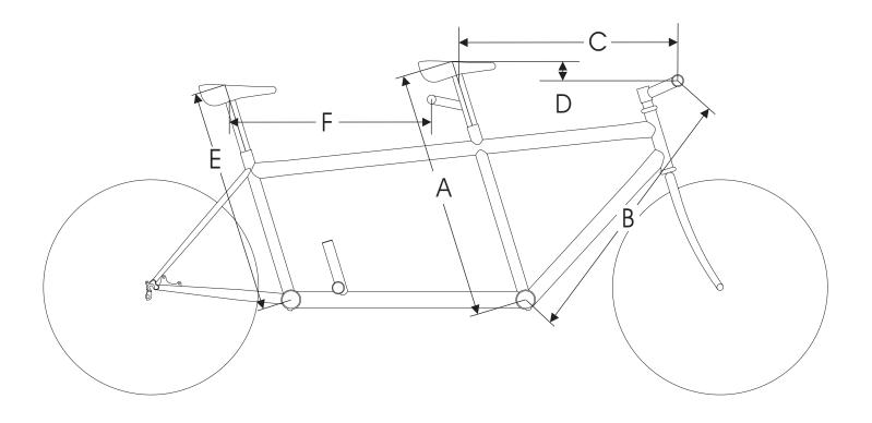
A) Measure from the top of the saddle to the centerline of the crank spindle. be sure to measure along the seat tube (at the same angle).
